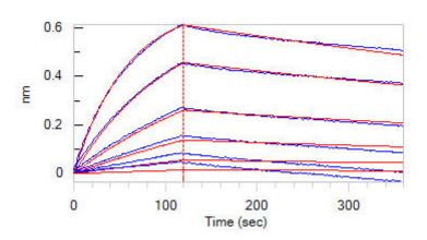
Loaded Anti-Fusion Protein Antibody, Human IgG1 (5B3) on AHC Biosensor, can bind Nipah virus Pre-Fusion glycoprotein, His Tag (Cat. No. FUN-N52H3) with an affinity constant of 8.4 nM as determined in BLI assay (ForteBio Octet Red96e) (Routinely tested).
