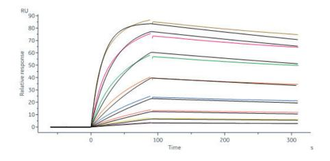
Bispecific T-cell Engager captured on Protein A Chip can bind Biotinylated Human CD3 epsilon, His,Avitag (Cat. No. CDE-H82E1) with an affinity constant of 2.62 nM as determined in a SPR assay (Biacore 8K) (Routinely tested).
